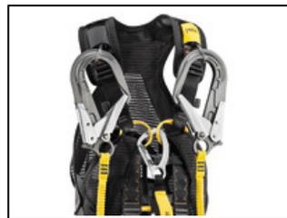
The MGO connectors on ABSORBICA fall arrest lanyards can be stowed on each shoulder strap. The user is thus unhindered by the lanyard, and the connectors stay within reach. In case of a fall, a system releases the MGO connectors to allow the absorber to be deployed.
