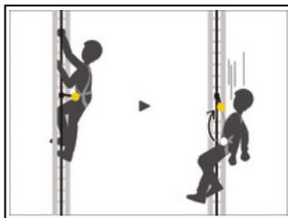
For vertical progression with a rail or cable-based fall protection system, the LADDER CLIMB attachment point allows for ventral attachment of the trolley. It distributes the load on the waistbelt and thus ensures optimal comfort during progression. In case of a fall, this attachment point automatically moves upward to a sternal position to ensure a vertical post-fall body position.
