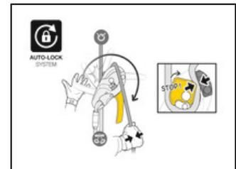
The AUTO-LOCK system allows users to easily position themselves at a work station without having to manipulate the handle or tie off the device: as soon as the user releases the handle, the rope is automatically locked in the device.
