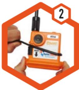
Slide the **ARMING SWITCH** down to the **[READY]** position until it clicks into place and ensure the **RESTRAINER TAB** is positioned in the gap above the **ARMING SWITCH**.
