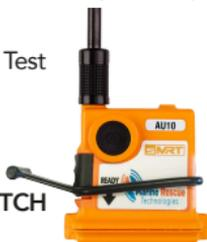
Ensure the **ARMING SWITCH** is in the **[OFF]** position.
