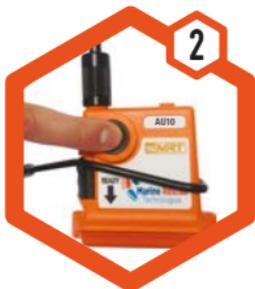
The sMRT AU10 can be manually activated by pressing the round rubber **ACTIVATION BUTTON**.
