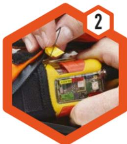
Remove the yellow **SWITCH LOCK** from the device and slide the red (V100) or black (V100X) **ARMING SWITCH** to the **[READY]** position. Both **LEDs** will turn solid blue for 5 seconds to confirm it is in **[READY]** mode.
