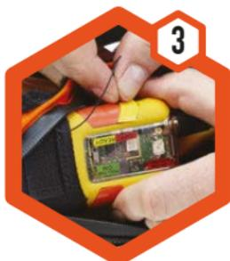
Reinsert the **SWITCH LOCK** above the **ARMING SWITCH** to lock it in the **[READY]** position.
